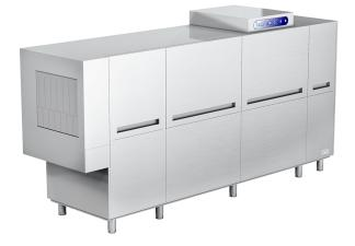
Width: 3070 mm Depth: 800 mm Height: 1580 mm Volume: 3.88 m<sup>3</sup> Rack dimensions: 500x500 mm Useful height: 410 Electrical power: 36.50 kW Electric power: 230 V/ 3 - 400 V / 3+N/ 50-60 Hz Racks/Hour: 160-215-270 Dishes/Hour: 2880-3870-4860
