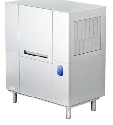
Width: 1200 mm Depth: 720 mm Height: 1380 mm Volume: 1.18 m<sup>3</sup> Rack dimensions: 500x500 mm Useful height: 430 Electrical power: 17.10 kW Electric power: 230 V/ 3 - 400 V / 3+N/ 50-60 Hz Racks/Hour: 85 Dishes/Hour: 1500 WAGP: Standard
