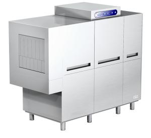
Width: 1870 mm Depth: 800 mm Height: 1580 mm Volume: 2.36 m<sup>3</sup> Rack dimensions: 500x500 mm Useful height: 410 Electrical power: 27.10 kW Electric power: 230 V/ 3 - 400 V / 3+N/ 50-60 Hz Racks/Hour: 90-135-180 Dishes/Hour: 1620-2430-3200
